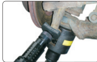
# 290 230 "VIBRO-IMPACT" ball joint separator
